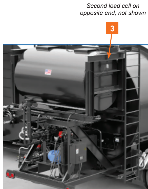
Horizontal Calibration Tank installed on a Heli-Tank
